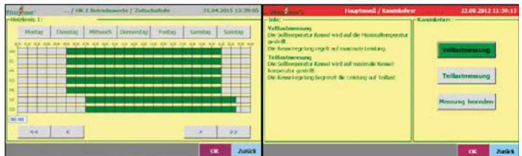
Simple setting of the timer for every heating circuit
