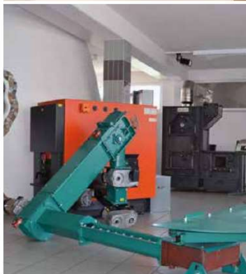
Discharge channel with inclined chain conveyor
